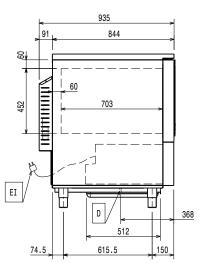
Drain Electrical inlet (power)
